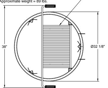
NOTE: CUSTOMER TO PROVIDE CONCRETE (RECOMMENDED)
