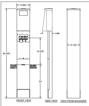
ETL-Certified, NEMA type 3R rainproof enclosure. One piece construction from G90 galvanized steel. All surfaces have electrostatic gray powder coated finish. 120/240 volt single phase, 125 Amp.
