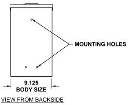
ETL-Certified, NEMA type 3R rainproof enclosure. One piece construction from G90 galvanized steel. All surfaces have electrostatic gray powder coated finish. 120/240 volt single phase, 125 Amp. Suitable for campground / RV and temporary service. Commercial quality receptacles. Tin plated copper stabs standard. All units factory wired.
