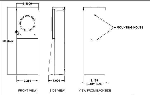
ETL-Certified, NEMA type 3R rainproof enclosure. One piece construction from G90 galvanized steel. All surfaces have electrostatic gray powder coated finish. 120/240 volt single phase, 125 Amp.
